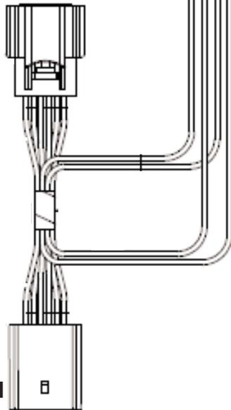
Connect to the accelerator pedal
