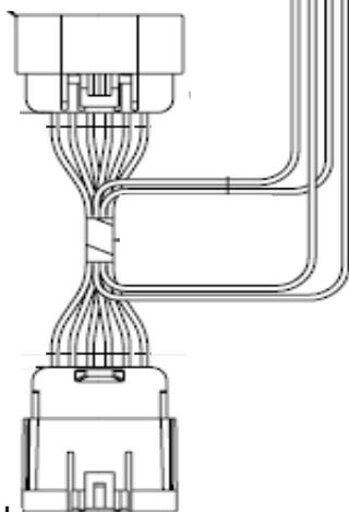
Connect to the accelerator pedal
