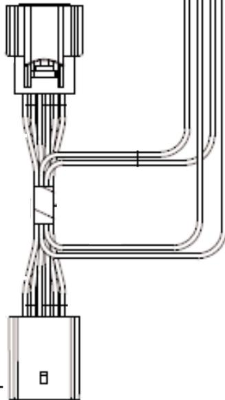
CONNECT TO THE ACCELERATOR PEDAL
