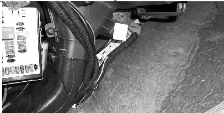
Remove the passenger-side panel from the center console and place the navigation interface module securely in front of the air conditioning system's ductwork connecting the **NAV\_IN** and **POWER** harness plugs leaving room for future access to the SD Card.
