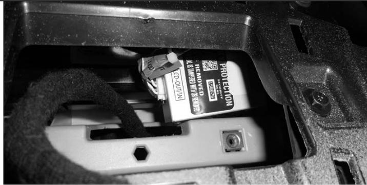
Connect the **OEM-IN** and **LCD-OUT/IN** harness plugs to the video switching control module. Connect the blue GVIF plug to the back of the factory touch screen.
