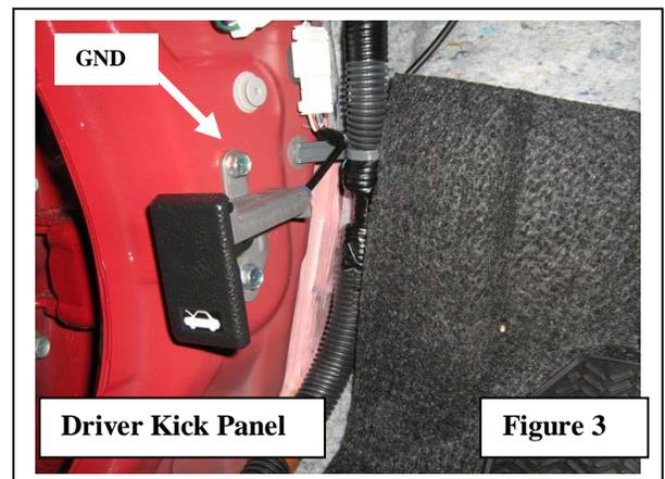
**B. 07-11 Honda Civic Wiring Connections (It is advisable use solder for all wiring connections)**
