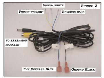
**NOTE:** IF REVERSE WIRE IS PRESENT IN VEHICLE CONNECTOR, REVERSE WIRES ARE NOT NEEDED FOR THIS APPLICATION
