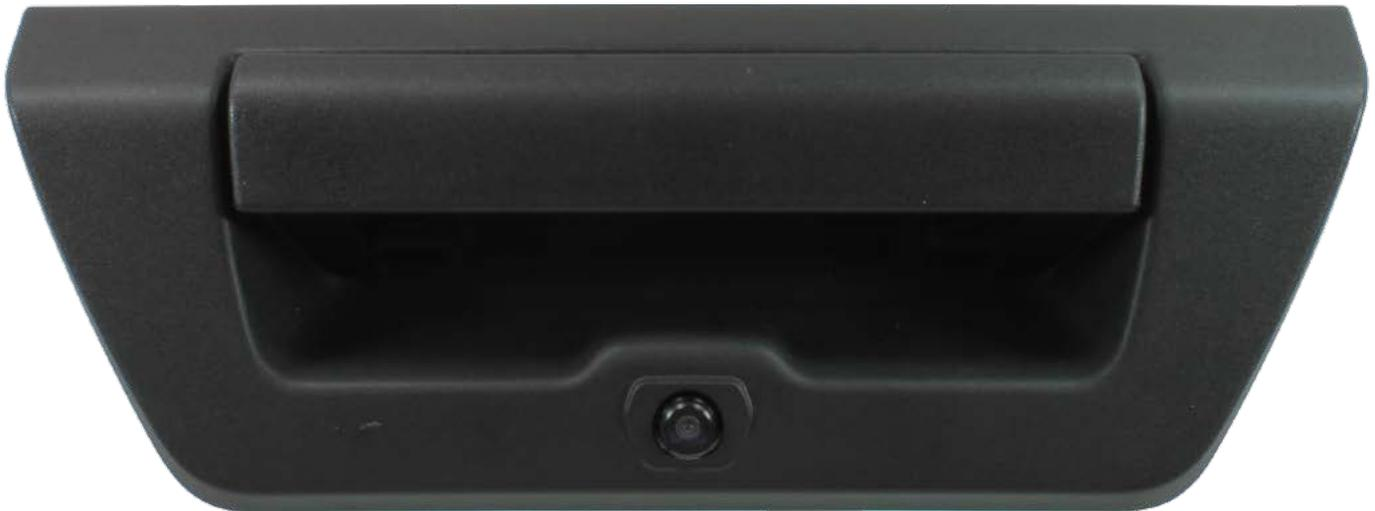
Available with screen interface module for Ford 4.2" display. Part number **250-8419-FDL15** includes module and latch camera.
