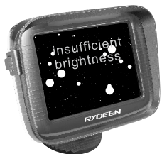
Image 3) The Camera may not have sufficient back light for it to capture a clear image. Check to make sure that the vehicle reverse lamps are turning On when the vehicle is shifted into reverse.
