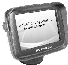
Image 1) The Camera may be receiving too much light into the lens. This is normally due to a poorly adjusted camera which may be capturing too much direct sunlight. Adjust camera so that it does not capture too much sunlight.
