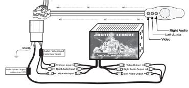
**Note:** This cable is intended for use in conjunction with an OS-4 to retain all safety and convenience systems. The vehicle should be equipped with a Panasonic Overhead LCD and IR system, in which the DVD player was part of the AM/FM/CD receiver. The OS-4 is needed to power the IR headphone system.
