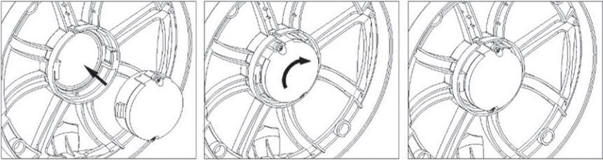
The above diagram shows the installation of the tweeter. Insert & rotate the tweeter clockwise. The removal of the tweeter is the opposite.
