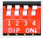
**Non-Navigation Radios:** Dipswitch 2 MUST be set in the **ON** (down) position for proper operation.
