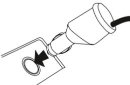
3. Plug the *PowerConnect* Power Adapter into the **red PWR** connector at the side of the *PowerConnect* Vehicle Dock.
