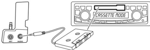
2. Insert the Cassette Adapter into the vehicle's cassette deck. You may need to turn on your vehicle's stereo system in order to do so.
