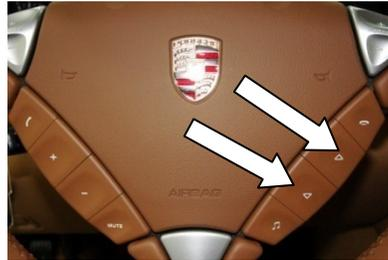
2. When **SERVICE** is displayed on the screen, press and hold the **up arrow** for **4 seconds** to program the PCM for reverse camera.
