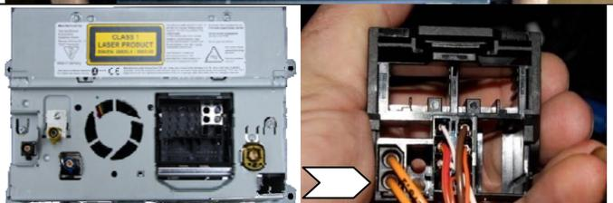
3. View of rear of radio and stock radio harness. Remove the fiber optic connector from the original harness by gently prying up on the locking tab with a pick tool.
