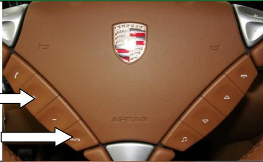
1. With the radio booted fully, Press and hold the **+ button** on the steering wheel.
