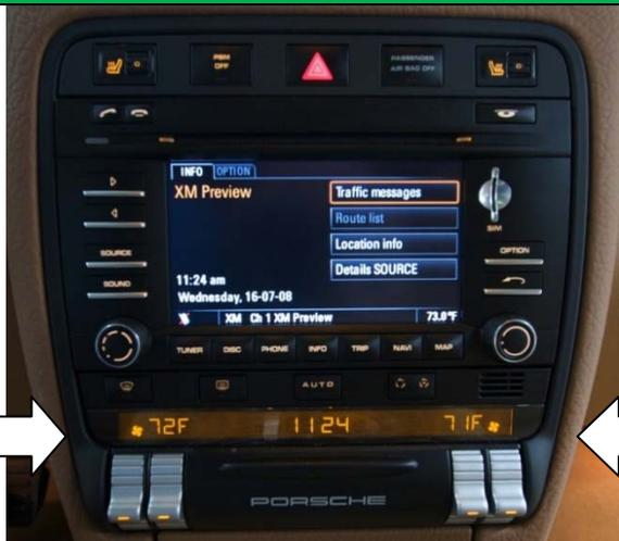
1. Insert a soft pry tool into the space between the lower black fascia piece and the lower side of the dash and gently pry the fascia towards the rear of the vehicle to release the mounting clips. Follow the fascia around either clockwise or counterclockwise to release the remainder of the mounting clips. Set aside the fascia.
