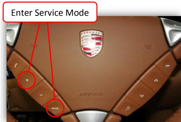
5. Press and hold the **UP ARROW** for **4 seconds** to program the PCM3 for satellite radio. *If this module is ever removed from the original vehicle you must first enter service mode and press the **DOWN ARROW** for 4 seconds to deprogram the original PCM3 BEFORE the module is removed. If this is not performed, the module will not work on any other vehicle!*
