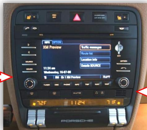
3. Remove (4x) Torx t20 screws that secure the radio into the sub-dash. Remove radio, disconnect all plugs and set the radio aside.
