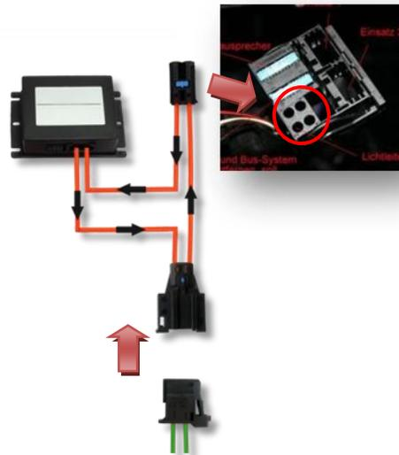
Vehicles without active fiber optics; which means without CDC, without phone or any other fiber optical components have optical wires at the navigation computer, but it is possible that the ring is not connected to the diagnostic connector in the glove compartment. In this case a connector bridge for optical wires is necessary.
