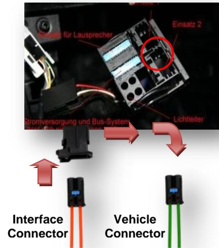
Connect the vehicle harness' fiber optical connector to the female fiber optical socket of the interface harness.
