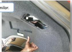
3. Disconnect the 2-pin plug connected to the factory logo handle:
