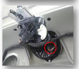
4. Remove (3x) Torx bolts that secure the factory VW logo to the trunk lid. Carefully pull the VW logo off of the trunk lid.
