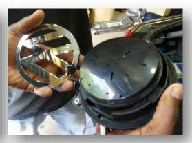
If the OEM chrome VW logo does not fit properly on the VW-CAM handle, it may be necessary to remove (pry off) the optional black oblong layer which comes connected by default on the VW-CAM.
