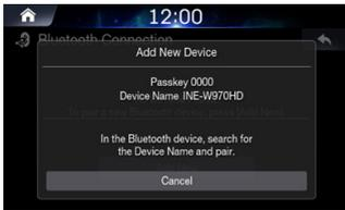
From the Bluetooth device, search for the AVN unit name and pair the device. When searching from the Bluetooth device, the AVN unit name is 'INE-W970HD' and the default passkey is '0000'.
